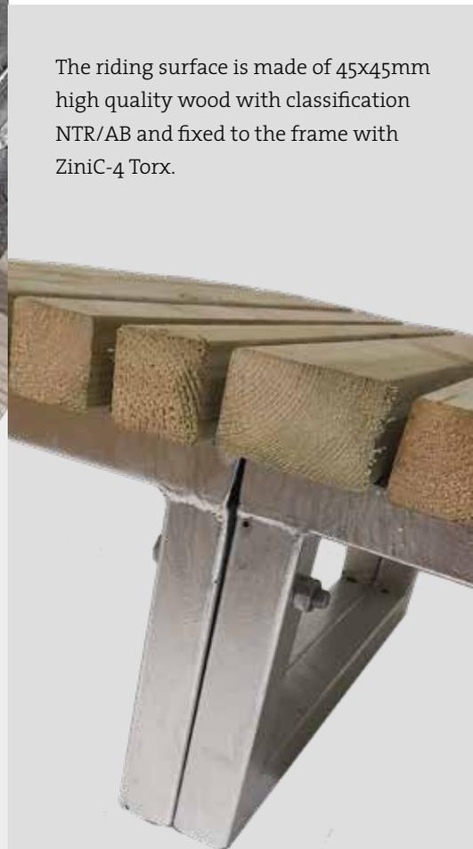
The riding surface is made of 45x45mm high quality wood with classification NTR/AB and fixed to the frame with ZiniC-4 Torx.
