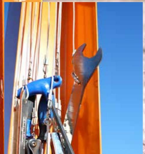
The tools - All necessary tools are securely attached to the stand with stainless steel cables and swivel connectors.
